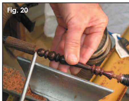
Fig. 20 Using a skew, carefully part off the scoop handle.
