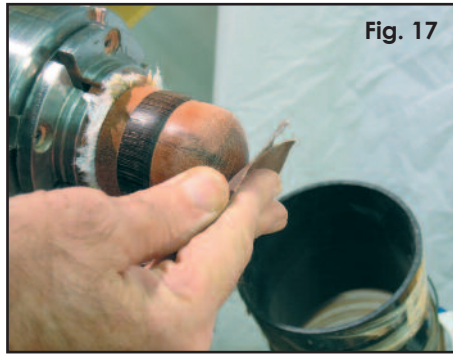
Fig. 17 If you have a set of small jaws, use them for finishing off the bottom.
