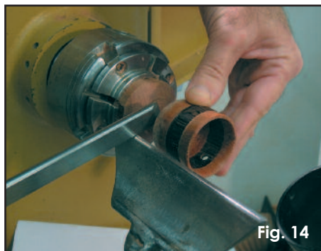
Carefully part off the scoop bowl with a skew.
