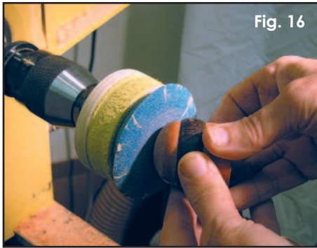
Fig. 16 A sanding mandrel with sanding disks can also be used to finish off the bottom.
